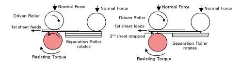
Reliable operation of a separation roller requires that its resisting torque be correctly specified and balanced with other forces. The frictional properties of the rollers and paper often change over time and with different operating conditions (such as humidity), so the resisting torque of the separation roller must be well controlled to ensure continued reliable paper separation.
