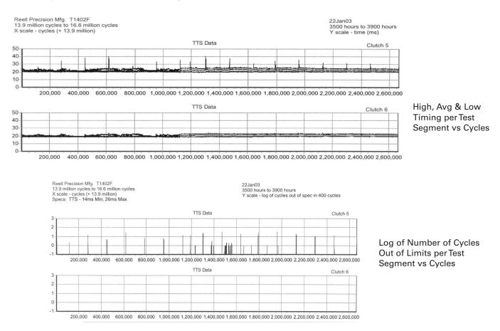
The actual cycle data can be plotted on screen and any area expanded to evaluate the extent of cycle-to-cycle variation at any place in the test. This chart shows the TTS results on clutch 5 with over 3000 hours and 15 million cycles as the fixture and clutch warm up after a long shut down.
