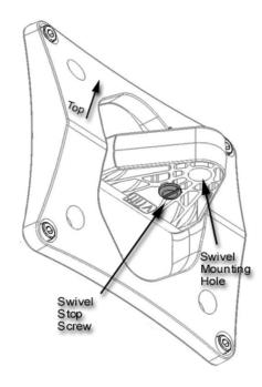
Horizontal motion can be limited by installing a #8 self tapping screw in the provided hole on the underside of the vTilt.
